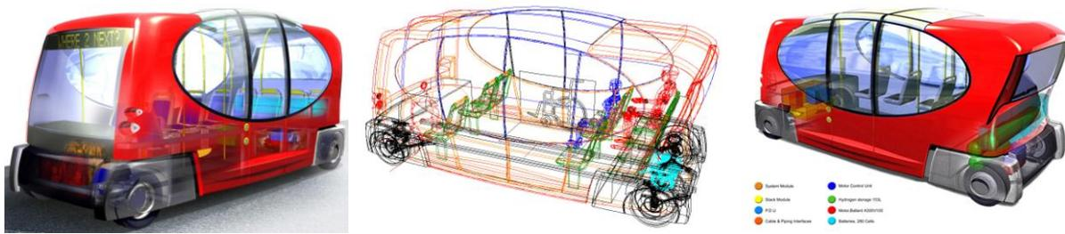
Figure 3a: Bio-fuel ICE      Figure 3b: Packaging design      Figure 3c: H<sub>2</sub> fuel cell version
